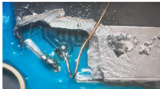
Figure 12. Conductor welded to the TAP.
