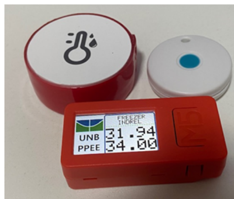
Figure 4: BLE connection between sensor and M5StickC
