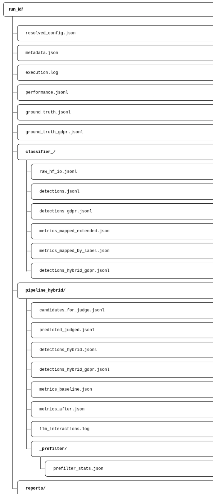
Figure II.5: Example directory structure of artifacts retained for a Pipeline 2 (hybrid) run, including base-line classifier outputs, candidate sets, judged outputs, and hybrid metrics.
